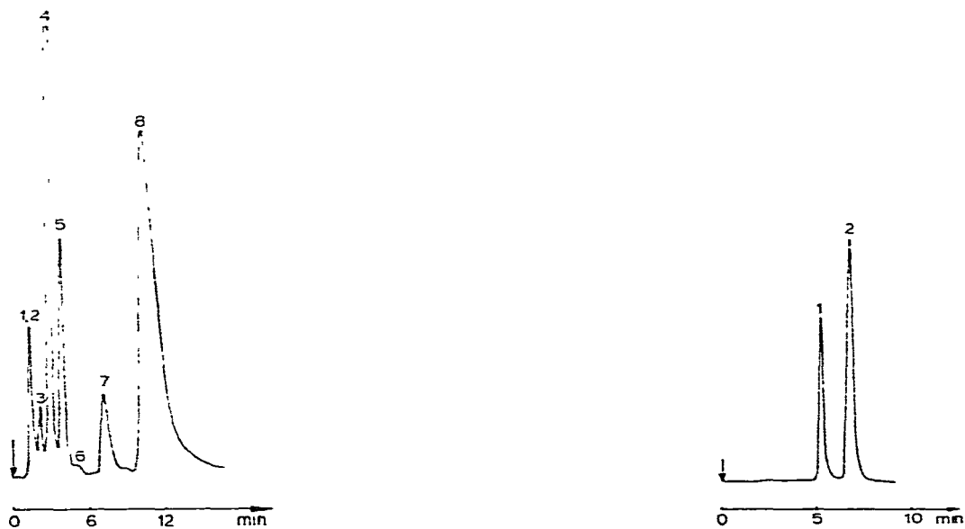
Fig. 2. Separation of vincanole and isovincanole in production mother liquor. Instrument, Varian 8500; column, MicroPak SI-10 ( 250 \times 2 mm I.D.); eluent; chloroform-ethanol (95:5); flow-rate, 20 ml/h; detection at 280 nm. Compounds: 1 = toluene; 3 = vincamone; 4 = vincamenine; 7 = isovincanole; 8 = vincanole; 2, 5, 6 = unknowns.
